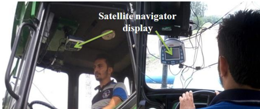
Figure 2. Satellite navigator fitted the tractor for without navigator and with navigator trial.
