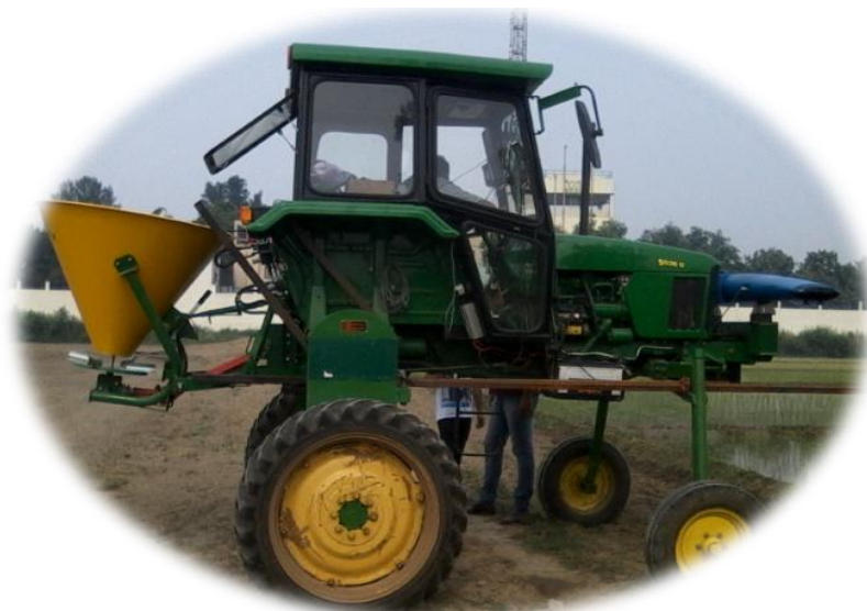
Figure 4. High clearance tractor (HCT) with fertilizer spreader used for urea spreading.
